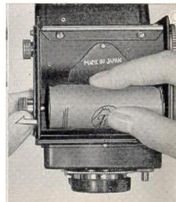
(5) Gently draw out the film leader. Thread the film leader into the wider slot of the Take-Up Spool in the Upper Film Chamber, then turn the Film Winding Knob. Make sure that the film leader is placed evenly.
